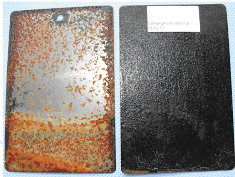
Fig 1: Left: untreated rusted steel plate; right: SCHWEGO ® inhibitor 6818 treated steel plate after reaction
