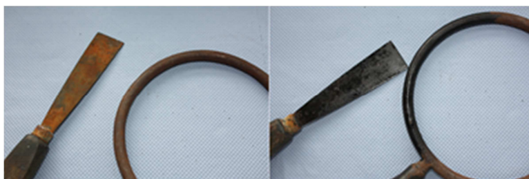
Fig 2: Rusty tools (left) and after treatment with SCHWEGO® inhibitor 6818
