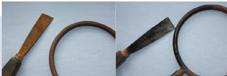
Fig 2: Rusted tools (left) and after treatment with SCHWEGO ® inhibitor 6818
